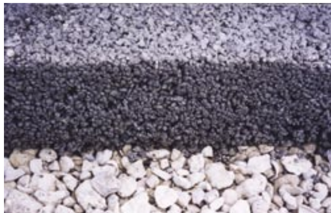
Fig. 1: Pervious concrete can be cast on an open-graded gravel base where subgrade soils are primarily clay
