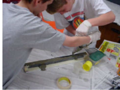
Students construct beams with varying amounts of mix water.
