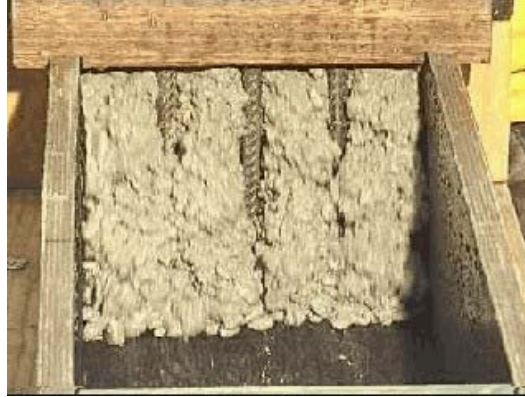
Figure 2.6: Flow through rebar in L-Box
